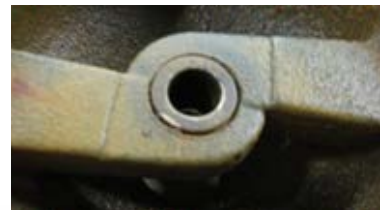
Above photo show discharge bearing after the destructive run-dry test.
