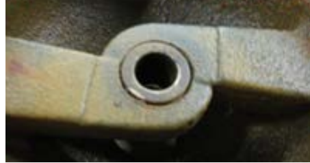
Above photo shows discharge bearing after the destructive run-dry test.
