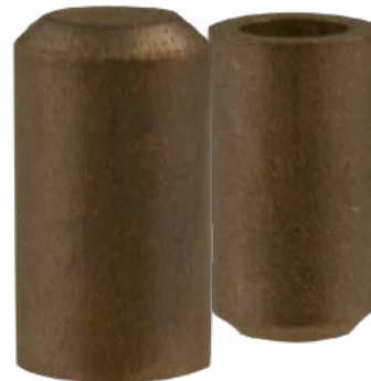
Above photo show discharge bearing after the destructive run-dry test.
