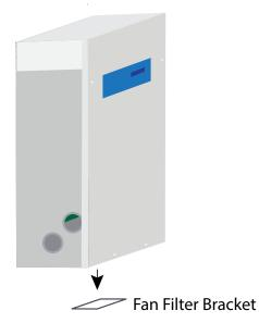
3. Place fan filter into filter bracket and snap the bracket back onto the bottom of the fan.
