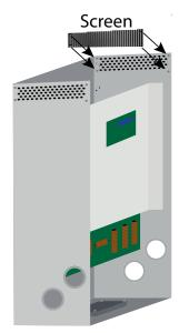
6. Line up the holes of one of the screen retainers with the mounting holes in the screen and the drive enclosure. Push the plastic rivets into the screen retainer holes.
