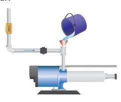
Pump only clean water. **DO NOT** pump water which contains sand, mud, silt or debris.
