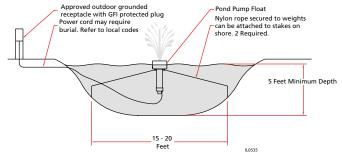
Figure 4: Typical Installation
