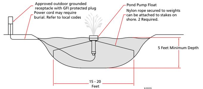
**Figure 4: Typical Installation**
